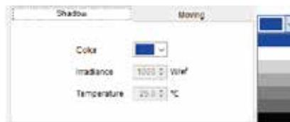
Set the irradiation and temperature parameters of clouds
