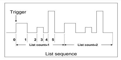
You can press the keys on the front panel of the electronic load to edit the sequence operation files, and trigger this sequence operation. Or you may directly recall existing sequence operation files to trigger the sequence operation. For example, when the DUT output voltage is 10V and the output current is 3A, after editing the sequence operation files under Constant Current (CC) mode, the steps for triggering sequence operation are as follows:
