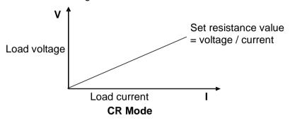
Fig. 3-3 Voltage-Current Relation Schema under CR Mode
