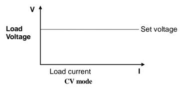
Fig. 3-2 Voltage-Current Relation Schema under CV Mode
