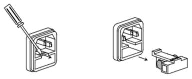
2) If the fuse is fused, please change fuse of same specification based on machine model. See the table blow for matching information of fuse and machine model.
